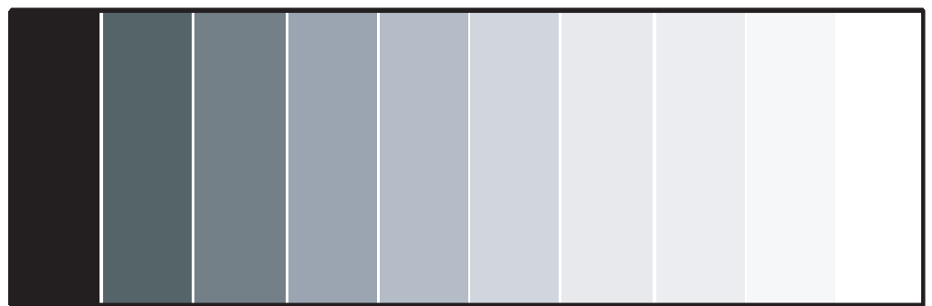
Figure 4-3. Typical Gray Bar Pattern for Adjusting Contrast
